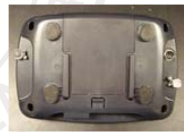
Indicator with wire security seal
