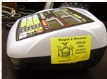
Indicator with paper security seal
